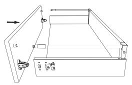
Assemble front panel on to the drawer.
