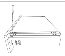
Tighten selftapping screws to fix bottom.
