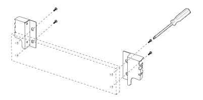
Assemble three drawer components by pressing the two sides against back panel.
