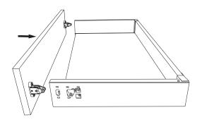
Assemble front panel on to the drawer.
