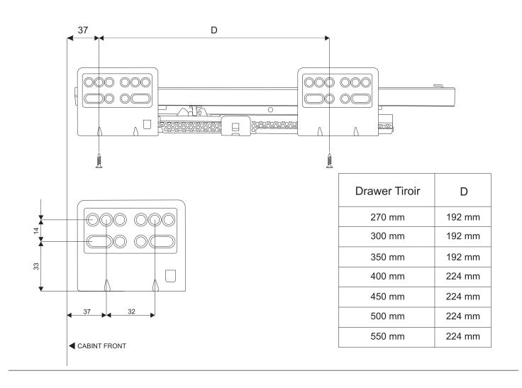
Assemble back connections to back panel.
