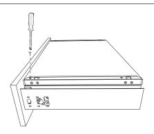
Tighten selftapping screws to fix bottom.
