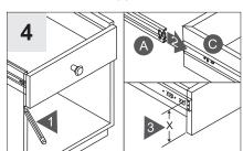
Determine drawer position. Mark bottom of the drawer front on the left and right sides. Place cabinet members (A) onto the drawer members (C). Measure "X".
