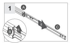
Press release the lever (B). Remove drawer member (C) from the Cabinet member (A).
