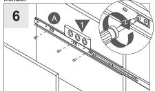
Make sure cabinet member (A) is level, secure with the screws. Repeat for the remaining cabinet member (A). Insert the drawer member (C) into the cabinet member (A) and close the drawer. Release member (B) will automatically locks.
