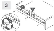
Make sure the drawer member (C) is level. Secure with screws. Repeat Steps 1-3 for the remaining drawer member
