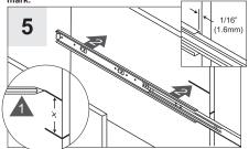
Mark "X" from the bottom of the mark. Repeat Step #1 to remove drawer member (C) from the Cabinet member (A). Align top of the cabinet member (A) with the mark, 1/16" form the front of the cabinet.
