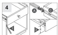
Determine drawer position. Mark bottom of the drawer front on the left and right sides. Place cabinet members (A) onto the drawer members (C). Measure "X".
