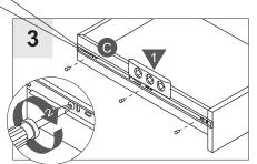
Make sure the drawer member (C) is level. Secure with screws. Repeat Steps 1-3 for the remaining drawer
