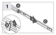
Press release the lever (B). Remove drawer member (C) from the Cabinet member (A).
