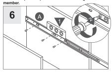
Make sure cabinet member (A) is level, secure with the screws. Repeat for the remaining cabinet member (A). Insert the drawer member (C) into the cabinet member (A) and close the drawer. Release member (B) will automatically locks.
