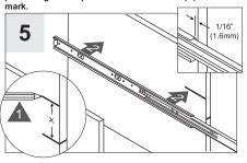
Mark "X" from the bottom of the mark. Repeat Step #1 to remove drawer member (C) from the Cabinet member (A). Align top of the cabinet member (A) with the mark, 1/16" form the front of the cabinet.
