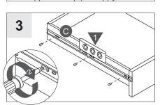
Make sure the drawer member (C) is level. Secure with screws. Repeat Steps 1-3 for the remaining drawer
