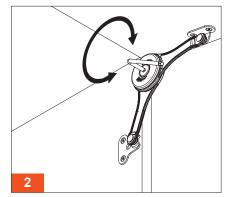
Adjust with allen key friction force according to flap door according to flap door dimension and weight using the adjusting screw.
