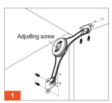
Fix always the brake leaving the adjusting screw always inside the cabinet.
