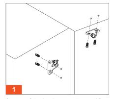
Screw on fixing brackets to cabinet and flap.
