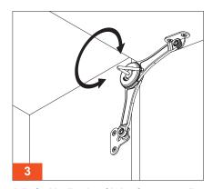
Adjust with allen key friction force according to flap door according to flap door dimension and weight using the adjusting screw.
