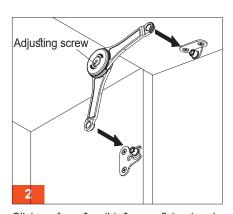
Click on free stop lid stay on fixing brackets to mount it leaving the adjusting screw always inside the cabinet.
