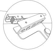
Lift the door up and assemble the mount plate with the lift fitting.
