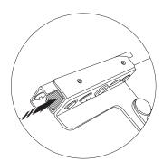
To disassemble press the clip button and lift the door.
